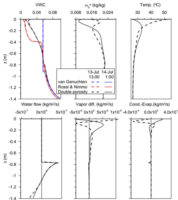
**Figure 7.** Simulated profiles during summer of VWC (volumetric water content),  $\omega_v^w$  (vapor mass fraction), temperature, fluxes of liquid water flow, vapor diffusion and condensation-evaporation of water. Positive fluxes are upward, negative downward. Condensation is positive and evaporation negative.
