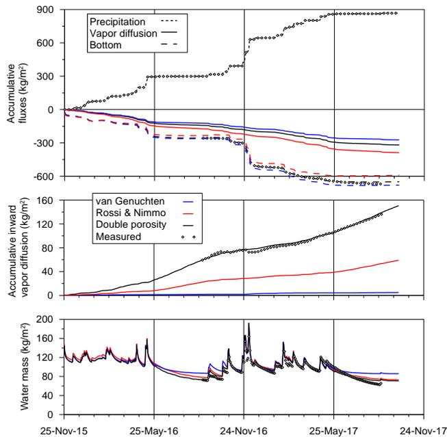
**Fig. 5.** Accumulative boundary fluxes (above and middle graph) and mass of water in the lysimeter (lower graph). Inflow is positive, outflow negative. Measured rainwater was used as input.
