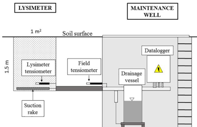
**Fig. 2.** Sketch of the Lysimeter.
