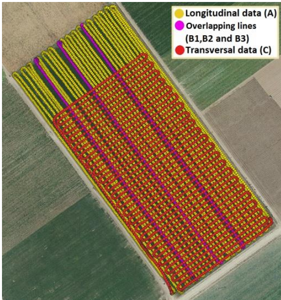
Fig. 2. Spatial layout of the ECa measurements used for the evaluation of the correction method. Measurements performed perpendicular to the drainage pipes are in yellow, in the direction of the drainage pipes in red and in magenta measurements in duplicated measurement lines.
